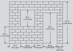
utilizing modular openings and opening locations (i.e., each dimension shown is evenly divisible by 8 in. (203 mm). By coordinating opening sizes and locations, the cells of hollow masonry units align (which facilitates the placement of vertical reinforcement and consolidation of grout), labor time
