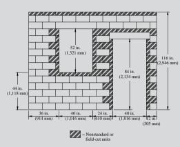
more costly compared to a similar structure employing a modular layout. Additionally, placing and consolidating grout in the reducedsize cores of the field-cut units may prove difficult. In this example, it is obvious the aesthetic impact non-modular layouts have on the final appearance of a structure. Not so obvi-
